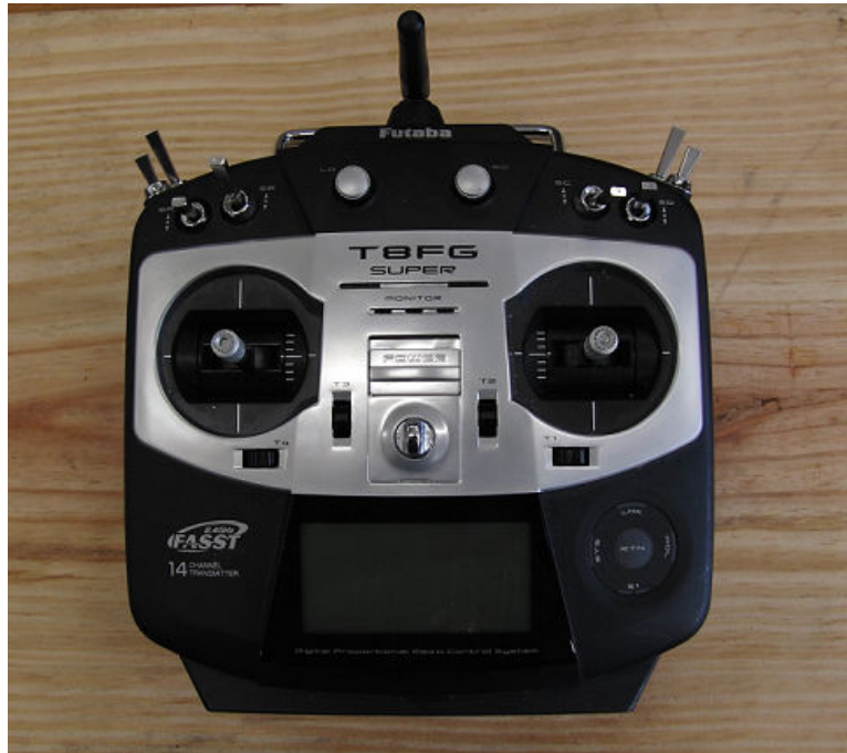
Figure 5.13: Remote control (Futaba T8FG Super) used to control HexaBull-2.
