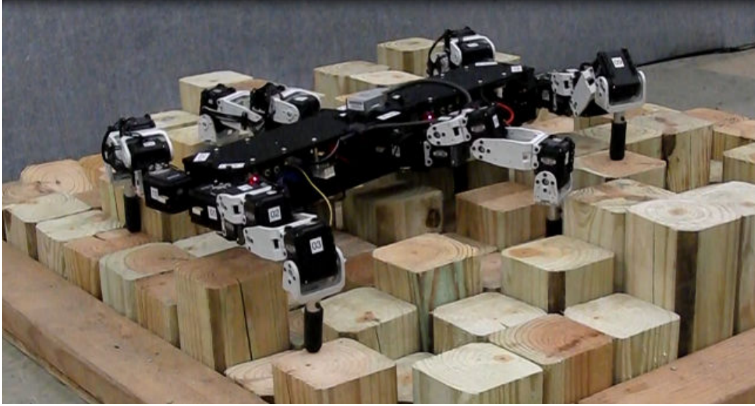
Figure 5.7: Experimental hexapod: HexaBull-1.
